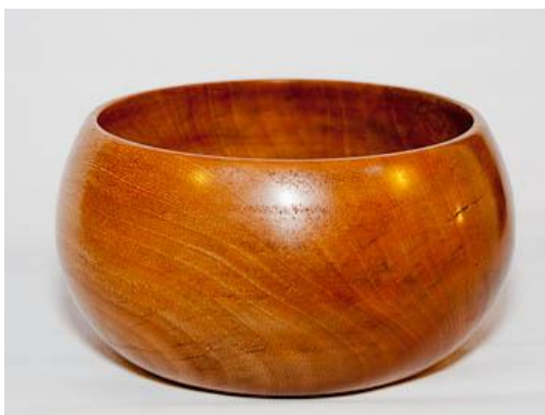
Johnny Alias showed a Small Salad Bowl made from Jackaranda finished with Sanding sealer and 50/50. Blank was mounted on a screw center, outside profile was turned. Blank was then reversed and mounted on a Vicmark chuck. Inside was hollowed using a homemade hollowing tool. Sanding sealer and 50/50 were then applied.
