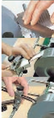
The Tormek wet grinder (above), and some of its accessory tool holders (left).
