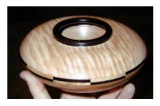
Before gluing the pieces in the rings, Al recommend to dry fit the pieces together. Hold them up to a light to check for gaps. Sand only the pieces that have a gap and then number the pieces with their position in the ring for final assembly. When gluing up the pieces into a ring, the glue must be applied evenly and thoroughly. Al uses quick release band clamps and
