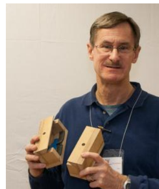
Mike Lanahan - Wood jaws for scroll chuck to hold mallet or gavel head while drilling the hole for the handle, and chamfering the edge of the hole.
