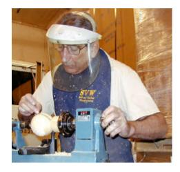
the lines. Rotate and repeat the process until the work is round. By rotating the work, you are removing the material by an averaging method, which tends to a near perfect sphere. The sanding is done in the exact same way. Sand and rotate, sand and rotate, etc. You can see Bob's method by visiting his Web Site at <a href="http://home.pacbell.net/renrut">http://home.pacbell.net/renrut</a> and click on "project".
