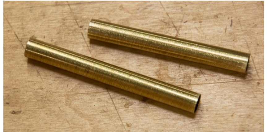
Both tubes are sanded and you can see the sanding marks on the tubes.
