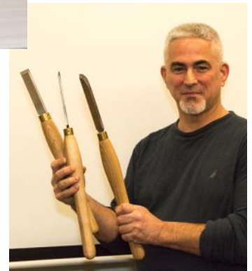
Brian Havens , Negative Rake Scrapers = less sanding.
