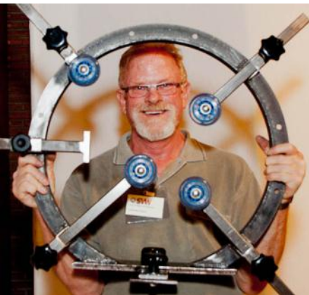
Lonnie Hurst - Jeff Nicol Style Steady Rest - Built and welded but not finished yet
