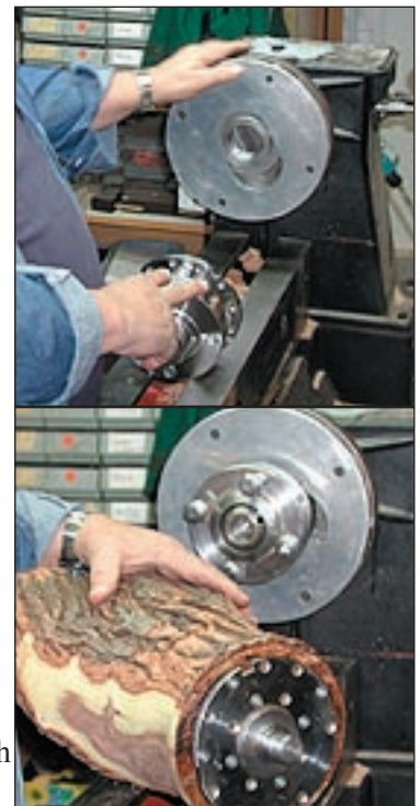
Above, two views of the McNaughton eccentric faceplate with accessory swash plate and faceplate. Below, Rich assembles Cole jaws on his Vicmarc chuck.
