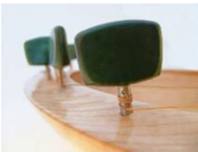
Photo 5. The strings pass over the wall at one end only in the simpler models. The steel tuning pins have maple thumb heads fitted shaped and stained so that the tuning system is part of the overall sculpture of the piece.
